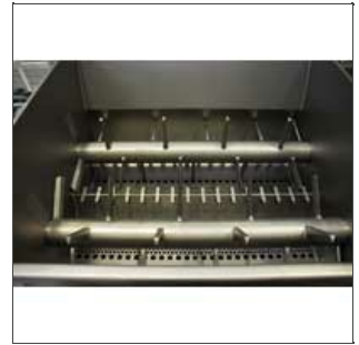
Shaft of the tank
