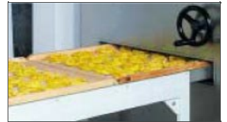
Detail of nested pasta in pre-dryer infeed
