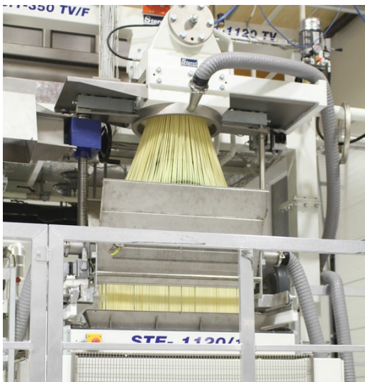
Application of STE 1120 on Omnia line with "mushroom head" spreader
