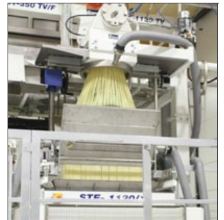
Application of STE 1120 on Omnia line with "mushroom head" spreader
