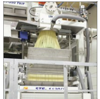
Application of STE 1120 on Omnia line with "mushroom head" spreading machine
