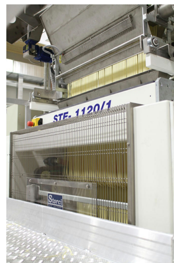
Application of spreading machine STE 1120 on Omnia line
