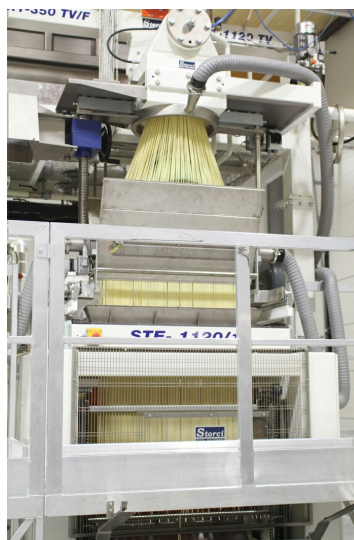
Application of spreading machine STE 1120 on Omnia line with "mushroom head" spreader
