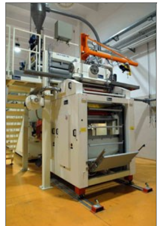
Application of STE 1120 FB on long-cut pasta line 130.1-1120/1 TV
